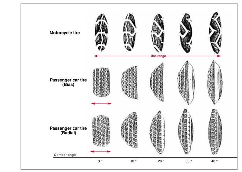
Motorcycle tires have acrown contour and basic construction which produces a minimal change in contact area when turnig.
