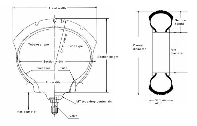
The simensions of a motorcycle tire are indicated here.In contrast to other types of tires,the tread width of motorcycle tires is normally wider than the section width.The section width included in the size marking of tires.A tire marked "120/90-18" means that the section width of the tire is 120 mm.
